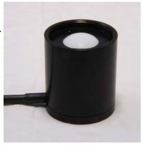
The UVB sensor PMA 2101 biologically-weighted erythema gives an accurate measurement of ultraviolet radiation from sunlight or artificial light sources, also called sunburning UV radiation (SUV). Its spectral response follows closely the erythema action spectrum. The detector has angular response very close to an ideal cosine function (Lambertian response) making it suitable for measurements of diffuse radiation or radiation generated by extended sources.
